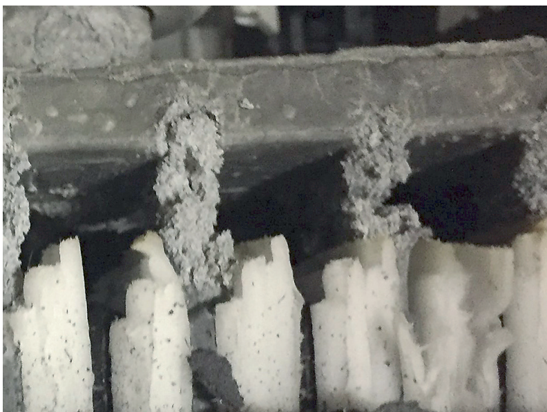
Fig 4: Severe negative tab failure, found upon dissection after initial alert with borescope. You can see the negative post/pillar also is decaying.
