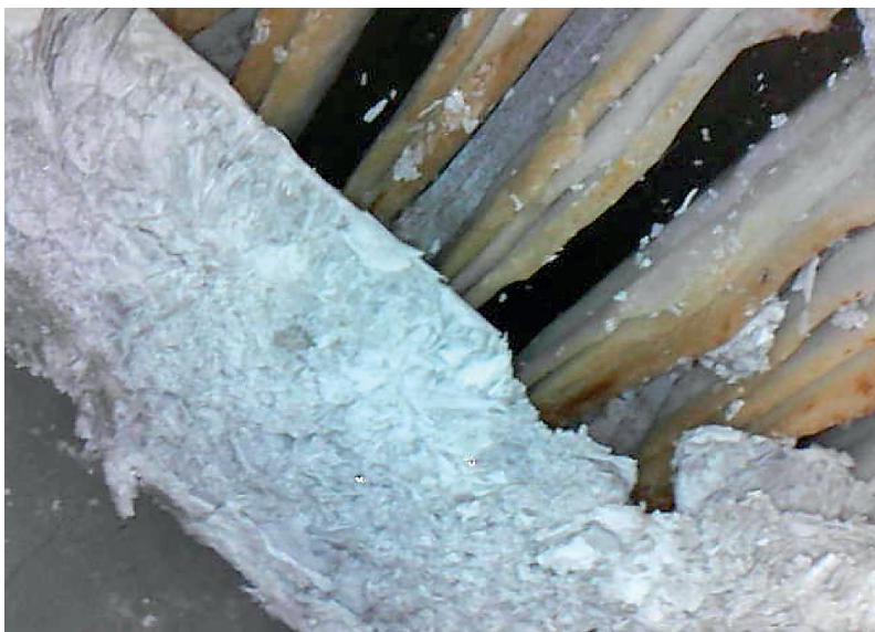
Fig 3: VRLA Negative bus breaking down observed with borescope. Battery on float.
