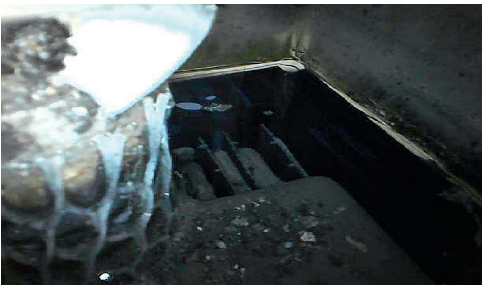
Fig 7: VLA internal positive post seal failure observed with borescope
