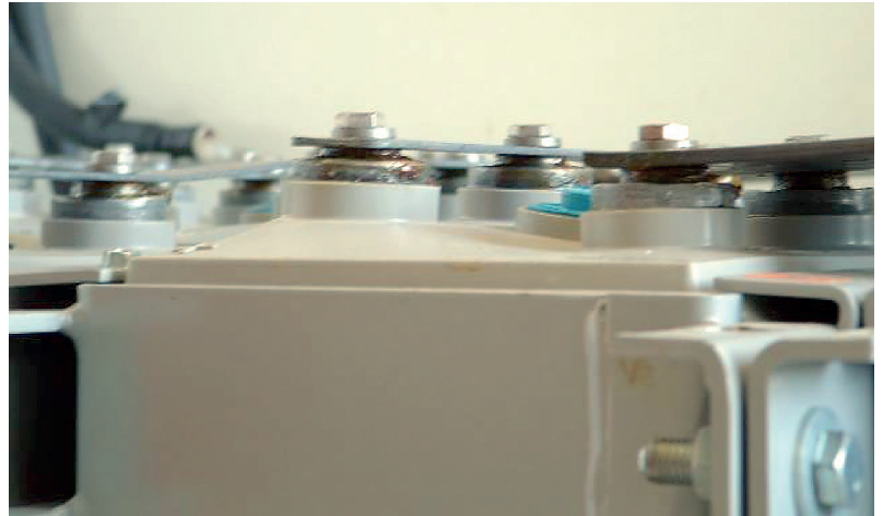
Fig 1: Extensive positive plate growth pushing cover upward around positive post.
