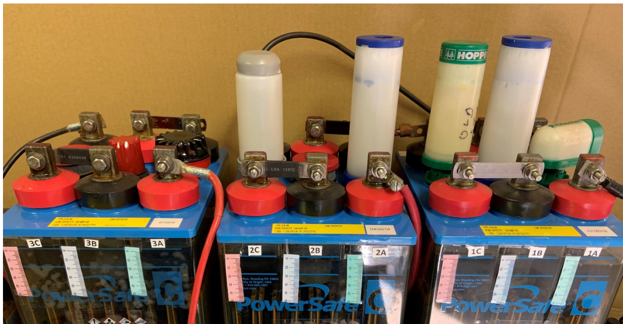
Exhibit 7. Picture of test arrangement with units with and without two-way valves.
