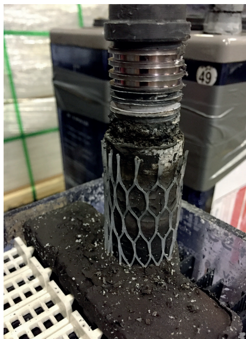
Fig 8: Condition of cell 53 post once the post-seal material was removed
