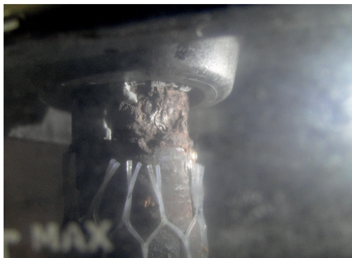
Fig 4: The brighter the light used, the easier it becomes to see some of the post seal faults
