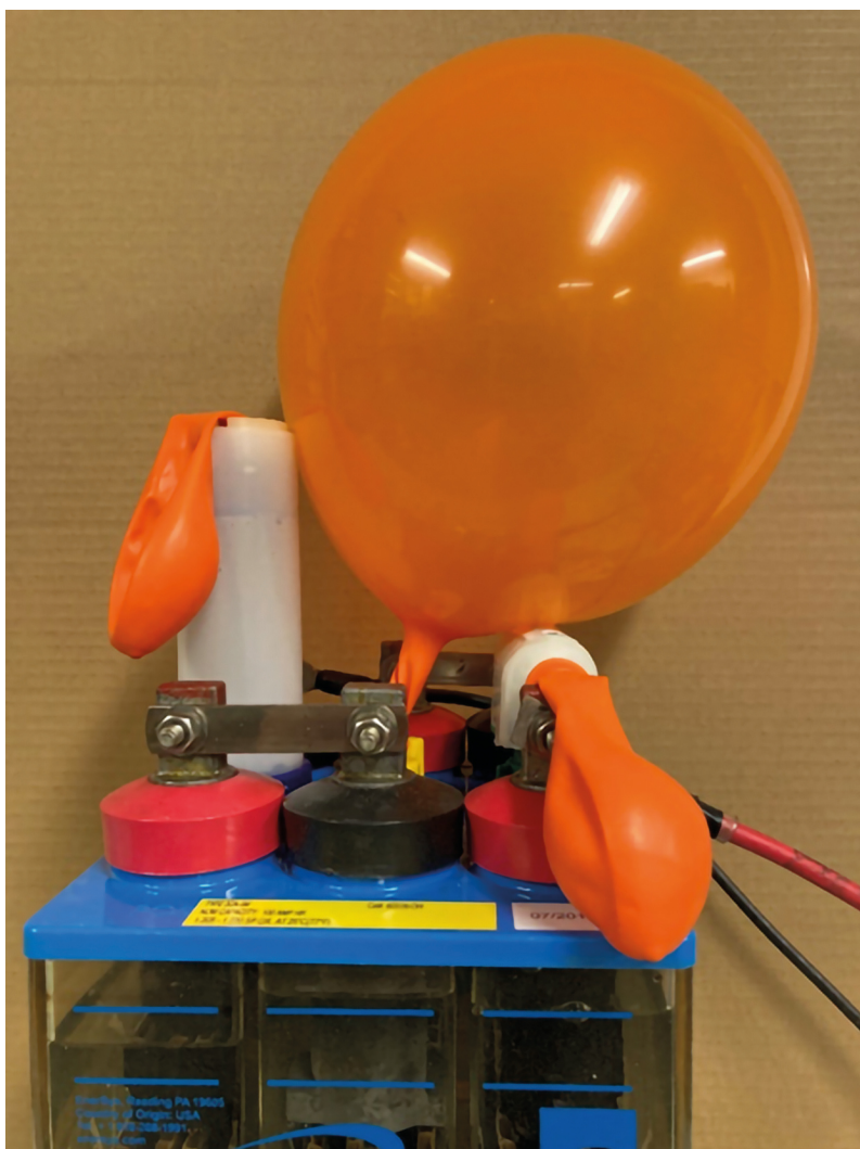
Fig 2: A visual demonstration of the amount of gas that recombiners can prevent from being released overnight
