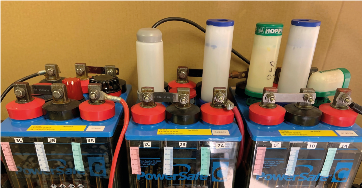
Fig 3: The test arrangement has units with and without two-way valves
