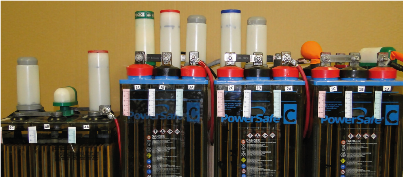
Fig 1: The test setup using recombiners from five different manufacturers
