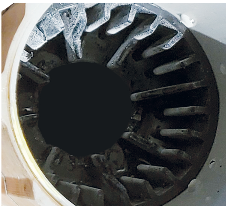
Pic 4: This picture shows the beginning of the catalyst core support structure melting, due to excessive internally generated heat due to the inability to control the amount of gas being recombined.
