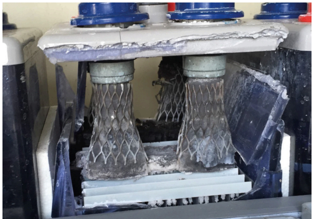
Fig 3: Cell that exploded when right rear positive post opened
