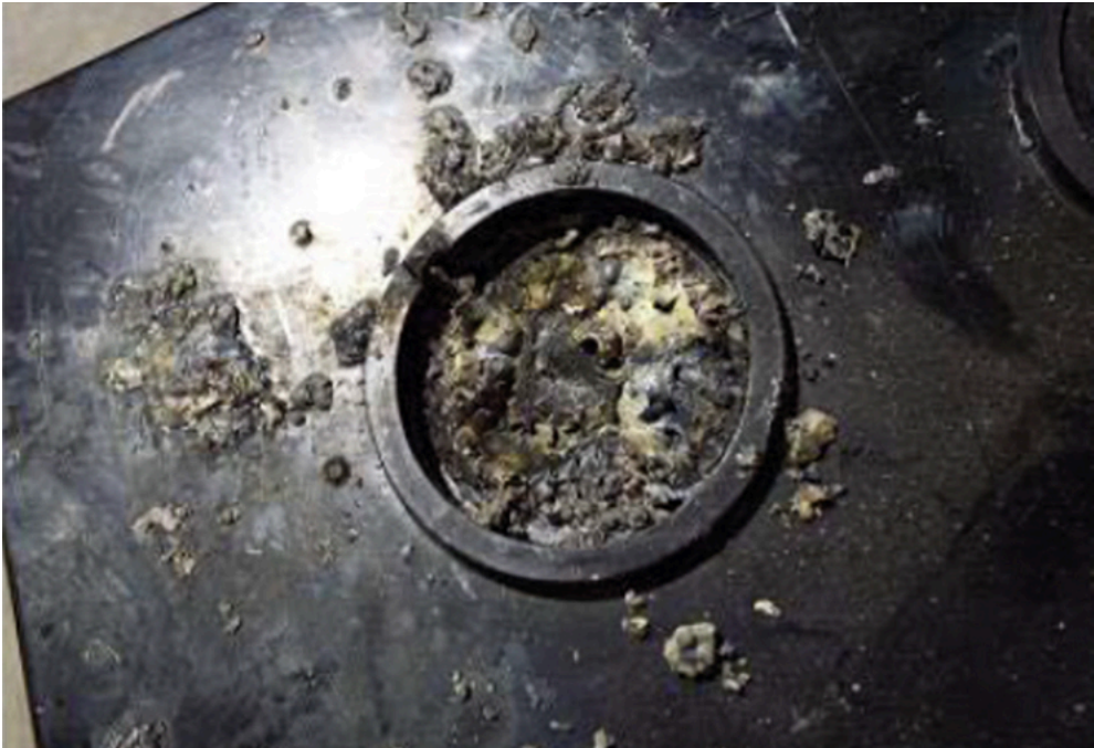
Fig 4: positive post that melted apart during the inrush part of testing
