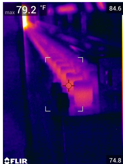
Figure 7 Nominal heating under normal conditions
